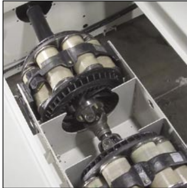
SuperFlow's dual eddy-current power absorbers are coupled with durable, low-maintenance driveshafts.
