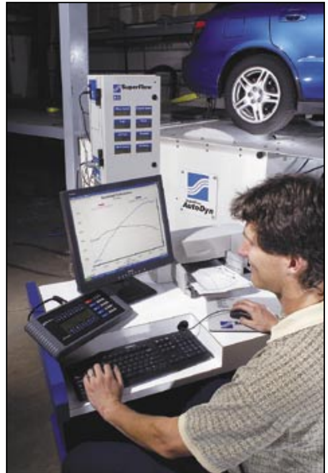
WinDyn helps you configure, execute, and analyze your AutoDyn tests. Sensor box shown with optional equipment.
