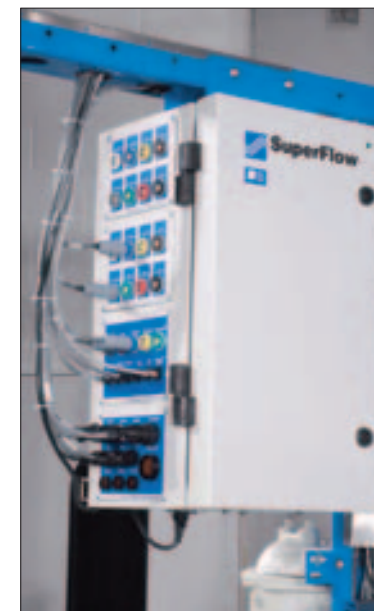
On NSCR systems, the sensor box can be mounted on the rail system. Sensor cables and pressure lines run through protected channels and exit near the sensor connections or near the sensor input panels. Color-coded and instrument-grade connectors simplify installation and help prevent connection errors.
